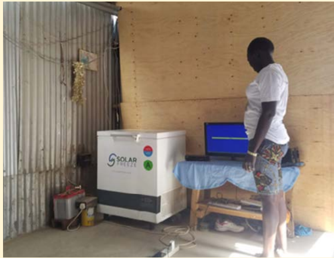
Besides using the Solar Freeze unit to run 2 businesses that store breast milk and cold water, Priscila has tapped the power from the 300 W solar panel to charge mobile phones, and operate a TV and radio.
